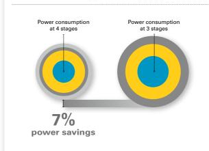
The ZD uses 4-stage configuration, which is 7% more efficient at compressing air than 3-stage configuration. The compression ratio is better and the interstage temperatures are lower. The results are impressive: energy is saved, reliability is enhanced, and maintenance costs are slashed.
