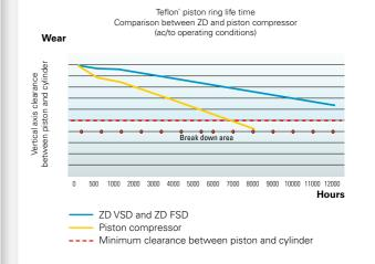
The ZD is equipped with a dryer at booster inlet to eliminate condensate. Compared to traditional piston technology, this saves energy and increases the life-time of moving parts (rings, packings, valves).
